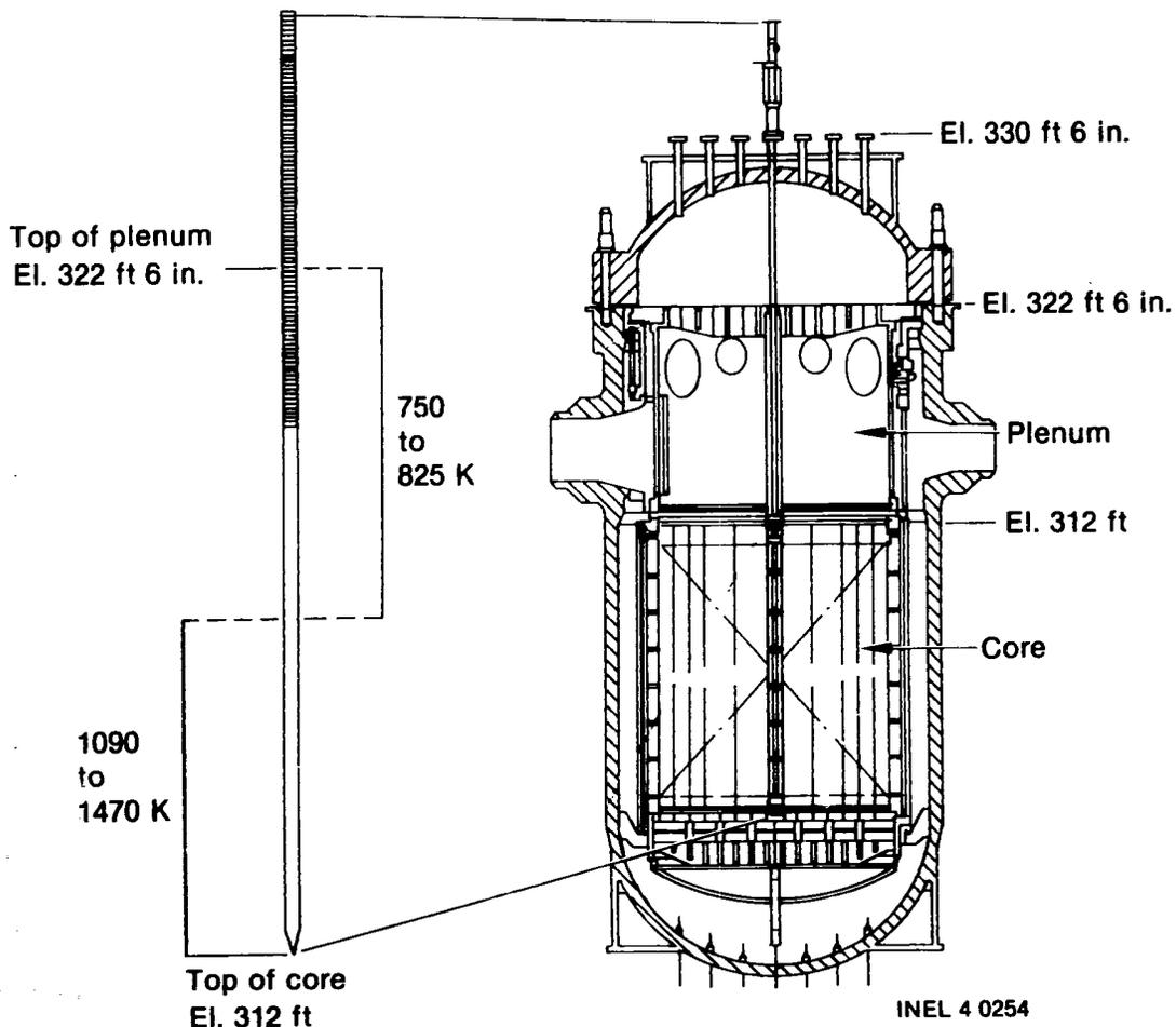
Figure 25. Approximate temperature ranges experienced by lower portion of the H-8 leadscrew during the accident.
