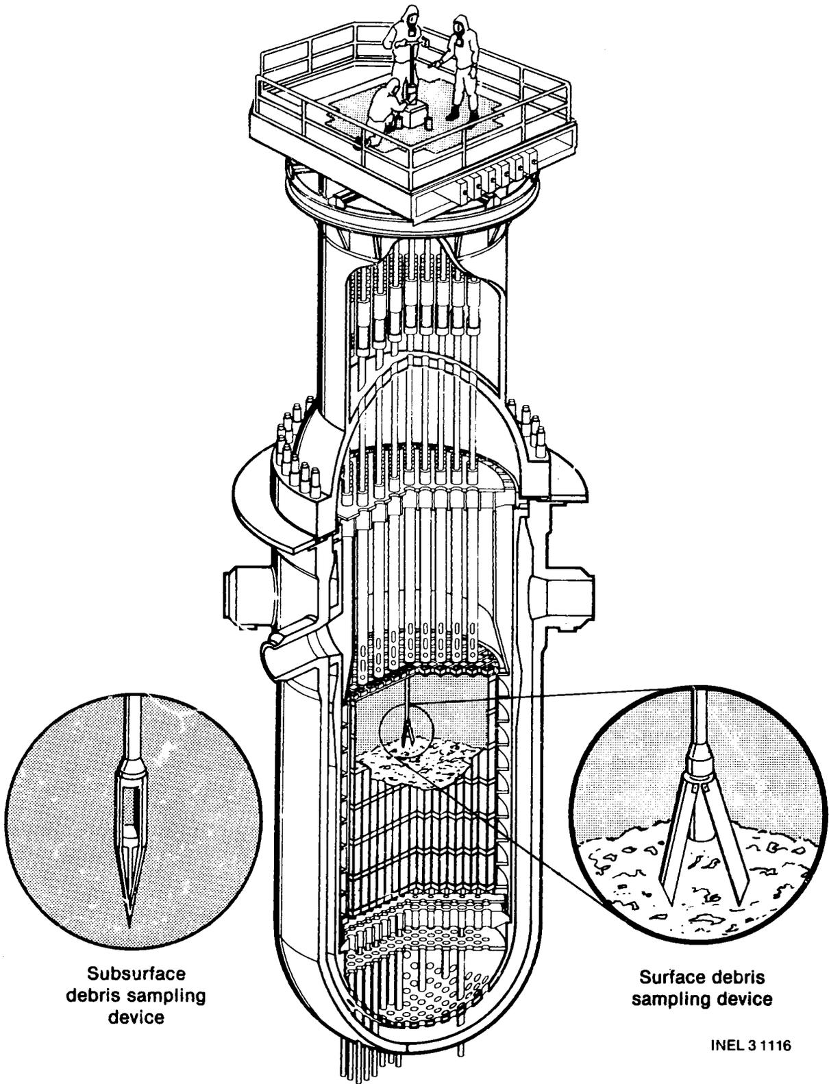
Figure 26. Core debris sampling at TMI-2 used two different sampling devices.
