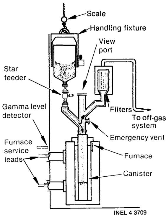
Figure 5. Zeolite vitrification system.
