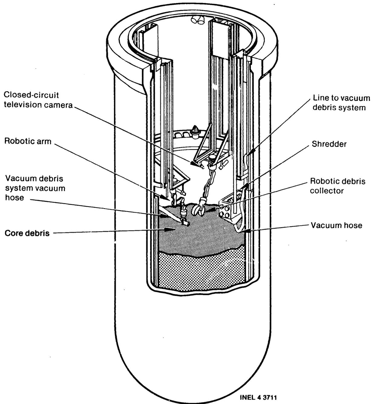
Figure 12. The Westinghouse Candidate Design System uses robotic arms to defuel the reactor vessel.
