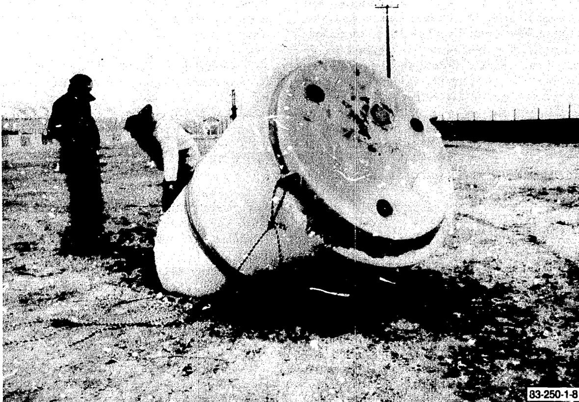
Figure 29. High Integrity Container shortly after drop test from 7.6 m, showing deep soil penetration and no damage to container.
