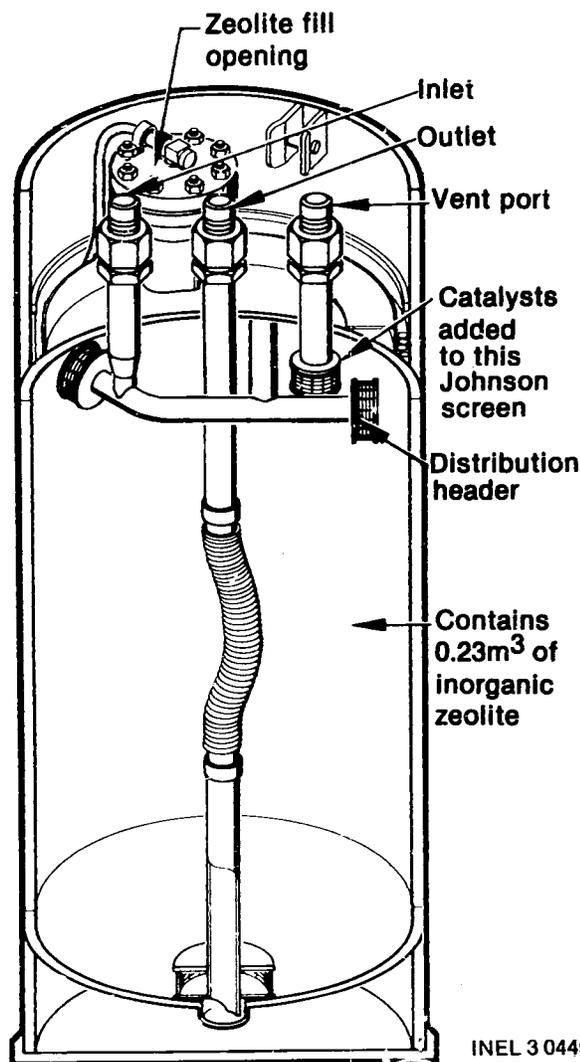
Figure 1. Cutaway view of an SDS liner showing Johnson Screen to which catalysts are added.
